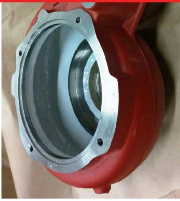
The additional cost of adding a protective coating to the volute and impeller was more cost effective than changing the substrate to an exotic alloy. The client was familiar with Belzona having used other Belzona coatings on other pumps. As the end user wanted to extend the life of an unprotected pump, the erosion resistance test data of 1331 and ease of application gave the client confidence that this was a long term solution.
